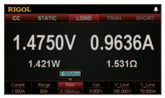
Current rising speed is defined as the speed of transition from one setting to another. You can set the actual transition time from one setting to another by changing the current rising speed. Adjustable current rising speed: 0.001 A/µs to 5 A/µs.
